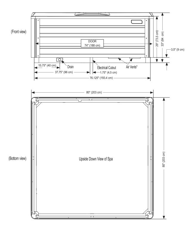
**NOTE: WATKINS WELLNESS** recommends that the **BEAM** be installed on a minimum 4" (10 cm) thick reinforced concrete pad or structurally sound deck able to support the "dead weight" found in the spa specification chart.
