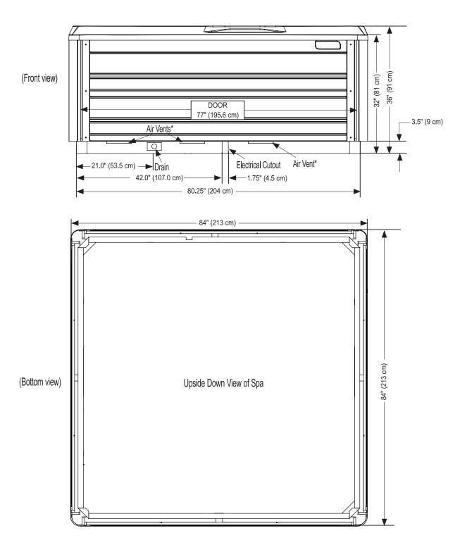
**NOTE: WATKINS WELLNESS** recommends that the **FLAIR** be installed on a minimum 4" (10 cm) thick reinforced concrete pad or structurally sound deck able to support the "dead weight" found in the spa specification chart.
