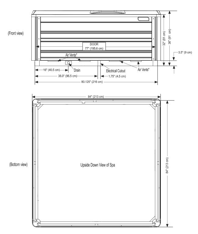
**NOTE: WATKINS WELLNESS** recommends that the **FLASH** be installed on a minimum 4" (10 cm) thick reinforced concrete pad or structurally sound deck able to support the "dead weight" found in the spa specification chart.
