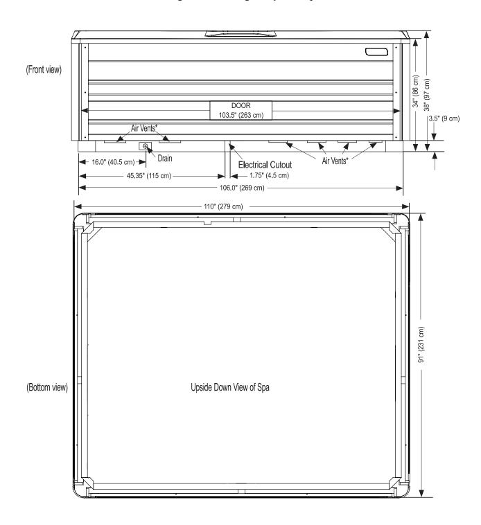
**NOTE: WATKINS WELLNESS** recommends that the **PRISM** be installed on a minimum 4" (10 cm) thick reinforced concrete pad or structurally sound deck able to support the "dead weight" found in the spa specification chart.
