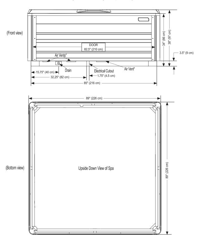
**NOTE: WATKINS WELLNESS** recommends that the **PULSE** be installed on a minimum 4" (10 cm) thick reinforced concrete pad or structurally sound deck able to support the "dead weight" found in the spa specification chart.
