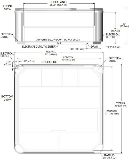
**NOTE: WATKINS WELLNESS** recommends that the PACE be installed on a minimum 4" (10.2 cm) thick reinforced concrete pad or structurally sound deck able to support the "dead weight" found in the spa specification chart.
