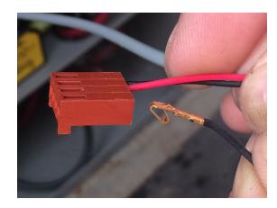
To reinstall wires, slide "finger" into harness with the finger curled down.
