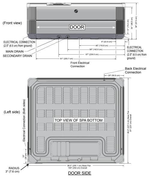
**NOTE: WATKINS WELLNESS** requires that the **ENVOY** be installed on a minimum 4" (10 cm) thick reinforced concrete pad or a deck that is able to withstand more than 120 lbs/ft<sup>2</sup> (570 kg/m<sup>2</sup>).
