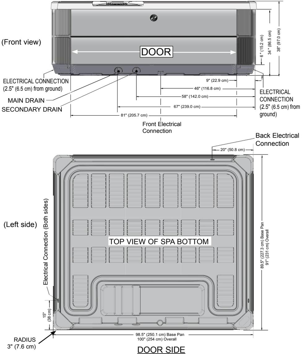
**NOTE: WATKINS WELLNESS** requires that the **GRANDEE** be installed on a minimum 4" (10 cm) thick reinforced concrete pad or a deck that is able to withstand more than 125 lbs/ft<sup>2</sup> (605 kg/m<sup>2</sup>).
