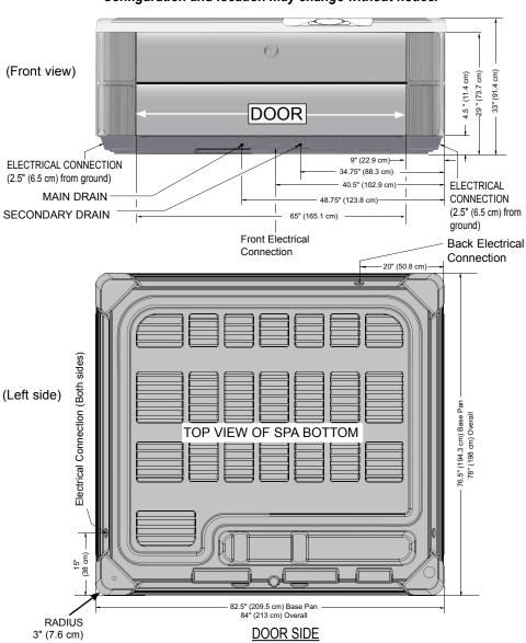
**NOTE: WATKINS WELLNESS** recommends that the **PRODIGY** be installed on a minimum 4" (10 cm) thick reinforced concrete pad or a deck that is able to withstand more than 130 lbs/ft² (620 kg/m²).
