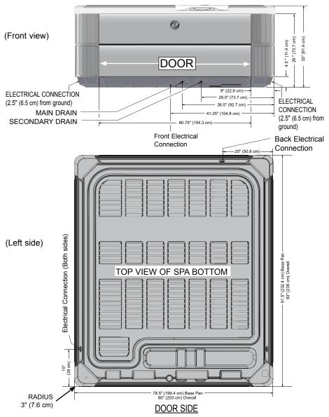
**NOTE: WATKINS WELLNESS** recommends that the **SOVEREIGN** be installed on a minimum 4" (10 cm) thick reinforced concrete pad or a deck that is able to withstand more than 115 lbs/ft<sup>2</sup> (555 kg/m<sup>2</sup>).
